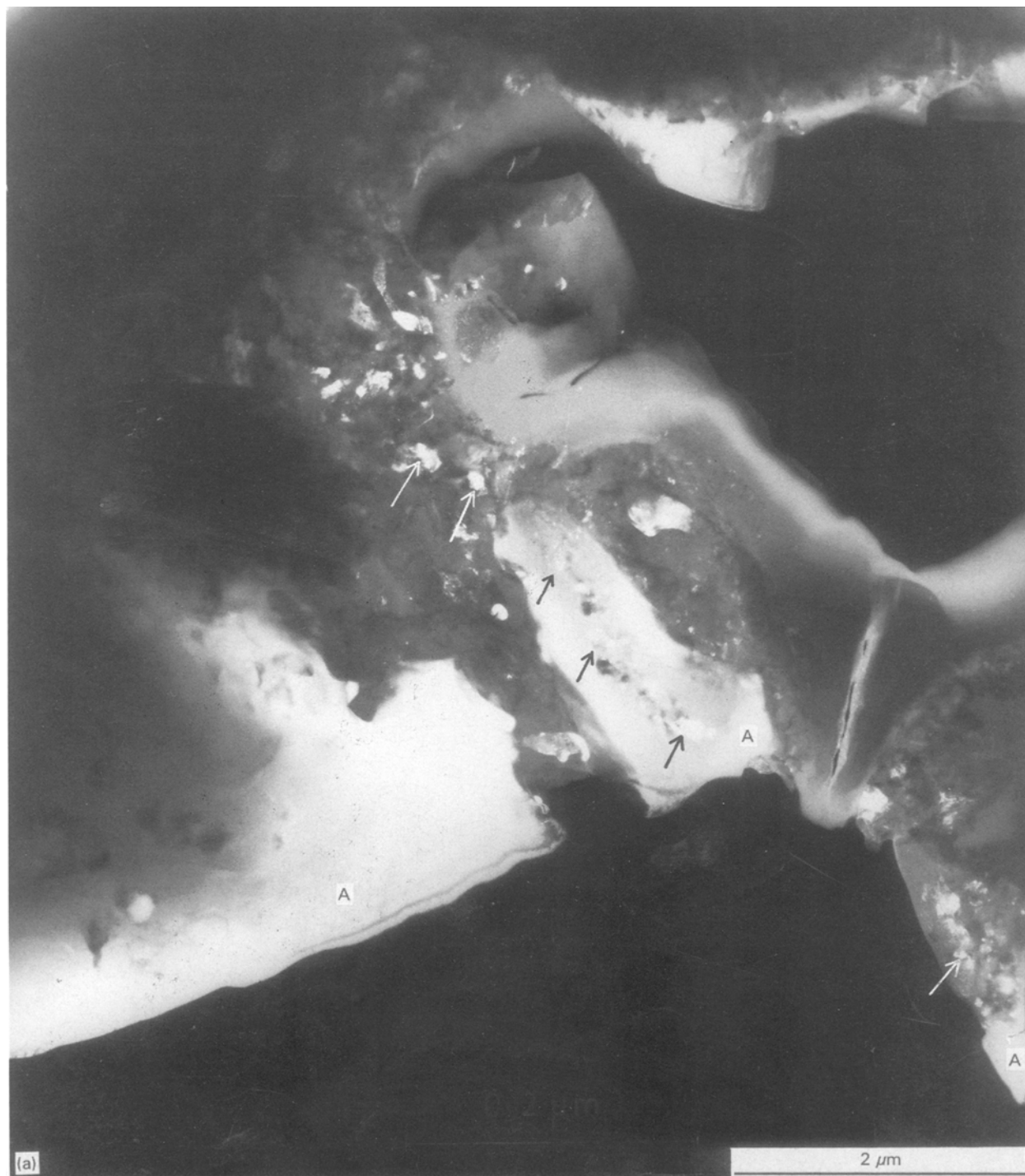
Figure 3 (a) Dark-field image of the surface region using an alumina reflection of a composite from Al–Mg–Si showing a fine microstructure (arrowed) interspersed in alumina “grains” (A). (b) Selected-area diffraction from (a). Because \text{MgO} and \text{MgAl}_2\text{O}_4 are fcc with lattice parameters of \sim 0.42 and 0.81 nm, respectively, many of the low-index diffraction rings overlap. The existence of both polycrystalline \text{MgO} and \text{MgAl}_2\text{O}_4 may be established by the three-arrowed rings which correspond to 4 4 0 (spinel), 2 2 0 ( \text{MgO} ) and 3 3 3/5 1 1 (spinel). The Al and \text{Al}_2\text{O}_3 are single crystalline over the dimensions of the selected-area aperture and yield spot patterns.
