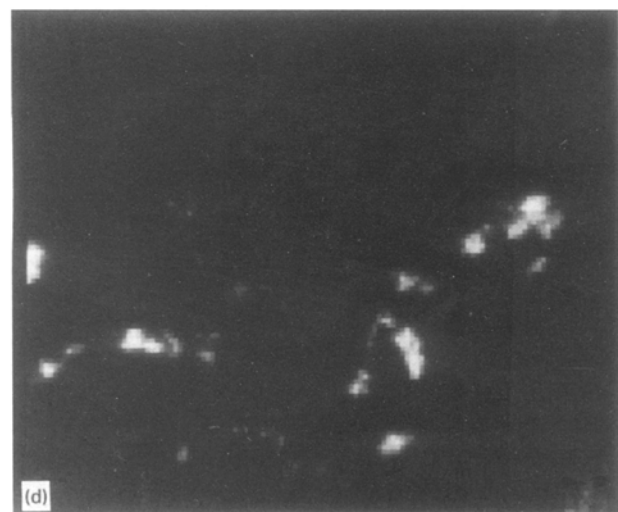
Figure 4 (a) Secondary electron image and (b–e) X-ray maps of the surface of a composite, showing the same field of view. Notice the large expanse at the top left (X) showing “particles” in a matrix. The dark contrast is characteristic of metal while the bright regions are magnesium-containing oxide. The chromium layer is shown dashed in (a), and as seen in the chromium X-ray map in (b–e), serves to define the positions of other elements with respect to the surface. (b) Al, (c) Mg, (d) Si, (e) Cr.
